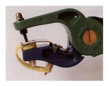
3. Be sure to completely squeeze the applicator so that the punch piece is completely imbedded in the collection cup.
